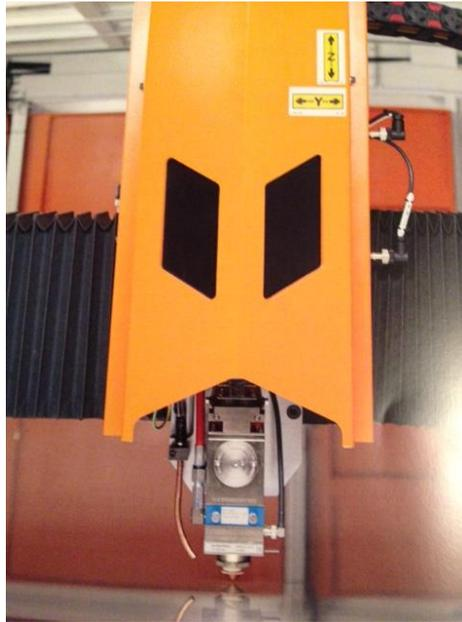
The Precitec Light cutting head is equipped with the quick manual focus adjustment to be changed with different material types and thickness.
