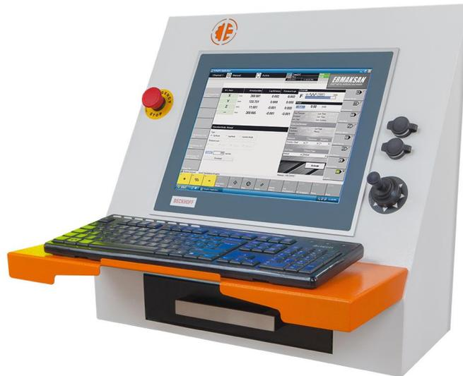
All cutting actions and axes movement input happen through the central located 15" Beckhoff 6202 Windows based touch screen controller & keyboard
